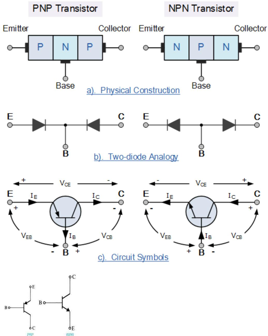
The direction of emitter arrow indicates direction of current flow.
