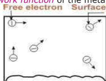
The metallic surface offers a barrier to free electrons and is known as *surface barrier*.
