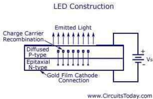
Fig. LED Construction
