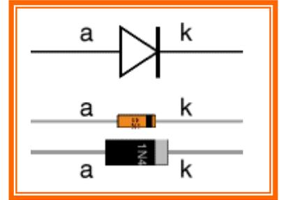
Small **signal diodes** can be damaged by heat when soldering, but the risk is small unless you are using a **germanium diode** (codes beginning OA...) in which case you should use a heat sink clipped to the lead between the joint and the diode body. A standard crocodile clip can be used as a heat sink.
