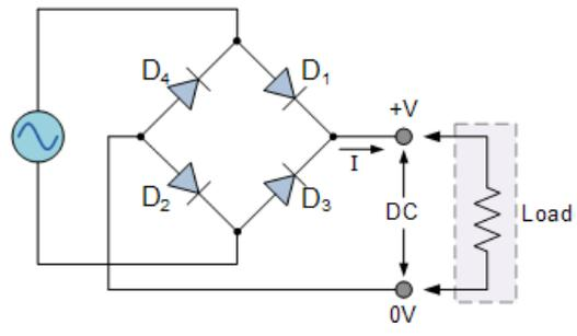
During the positive half cycle of the supply, diodes **D1** and **D2** conduct in series while diodes **D3** and **D4** are reverse biased and the current flows through the load as shown below.
