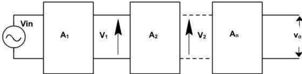
In a multistage of amplifier, a number of signal amplifier are connected in cascade arrangement i.e. o/p of first stage is connected to the i/p of the second stage through a suitable coupling device and so on. The purpose of coupling device is
