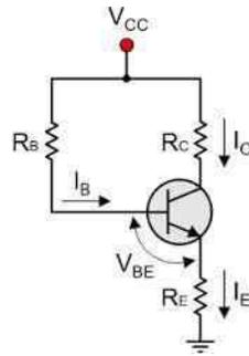
Circuit Operation of Base Bias Circuit : The required zero signal base current is provided by  $V_{CC}$  and it flows through  $R_B$ .
