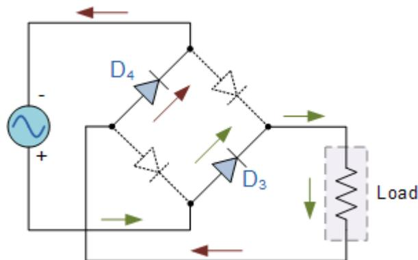
Max. rectifier Efficiency = Max. d.c. output power / a.c. input power =  $\eta = 81.2\%$
