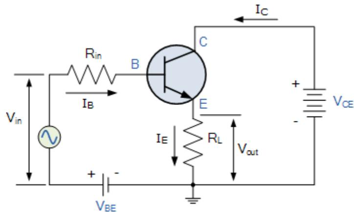
Working Principle: As the collector is at ac ground , the circuit is known as CC amplifier.
