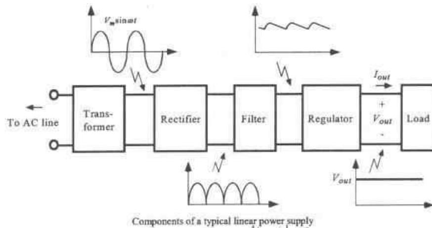
Working Principle: The output of power supply ( $V_{in}$ ) is fed to the voltage regulator which produces the final output ( $V_{load}$ ). The output voltage ( $V_{load}$ ) remains constant whether the load current changes or there are fluctuations in the AC input.
