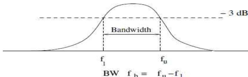
Where  $f_u$  is the upper cut-off frequency and  $f_l$  is the lower cut-off frequency.
