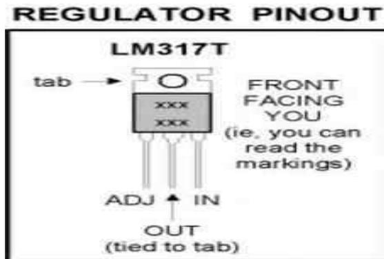
Pin-1 adjustable/variable , Pin-2  $V_{out}$  & Pin-3  $V_{in}$
