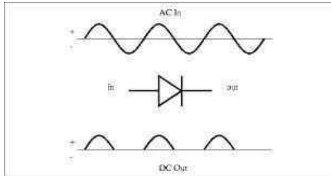
**Example-Diodes** : Diodes are useful electrical components for rectification purposes. Diodes are used in many applications like the following.
