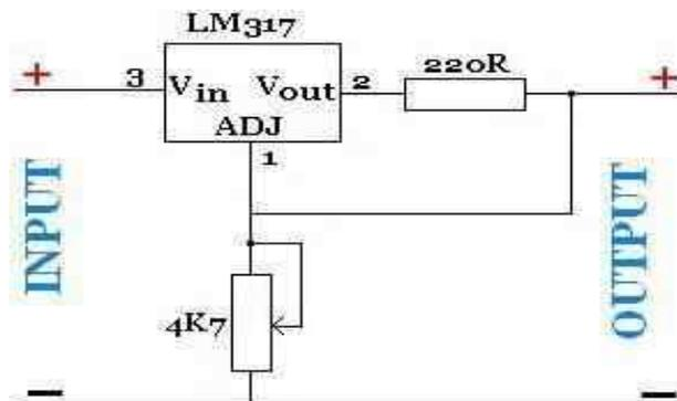
By varying the value of  $R_2$  the output voltage can be adjusted.
