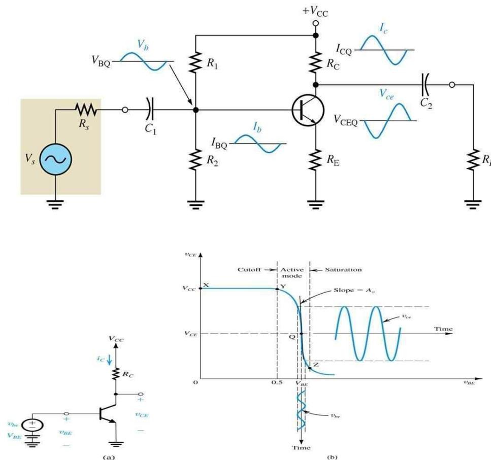
The above circuit shows the practical circuit of transistor amplifier with common emitter configuration. Resistance  $R_1$ ,  $R_2$  and  $R_E$  forms the biasing and stabilization circuit. The biasing circuit must establish a proper operating point otherwise a part of the negative half cycle of the signal may be cut off in the output. This circuit consists of three capacitors  $C_{in}$  or  $C_1$ ,  $C_E$ ,  $C_C$  or  $C_2$ .
